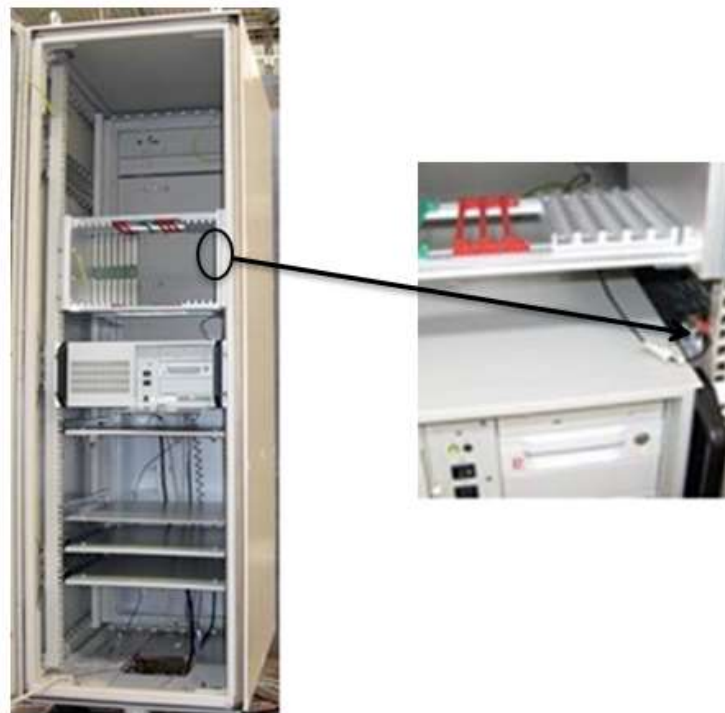
Figure 9-Inside of Cabinet Showing Sensor Measuring Acceleration
