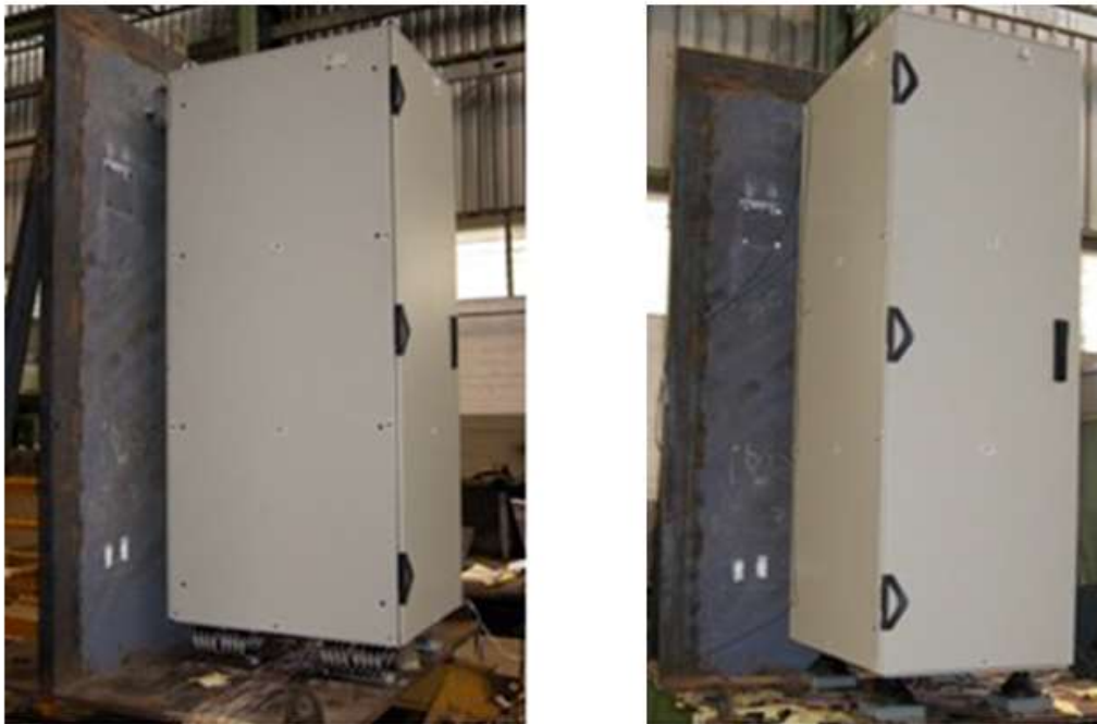
Figure 8-Test Setup on Wire Rope Isolators (Left) and Elastomeric Isolators (Right)
