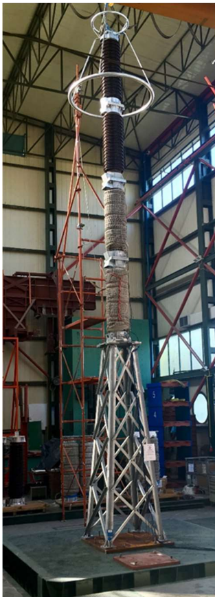
Figure 10. Test setups used of hard mounted case (left), elastically mounted case (right).
