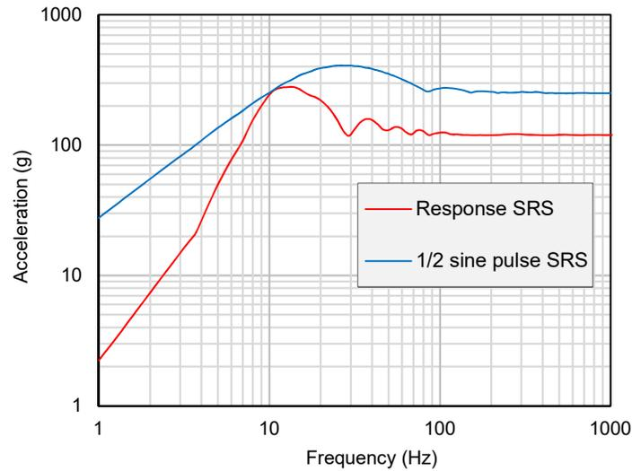
**Figure 12.** Example representation of the equivalent pulse input compared with the response SRS of the system
