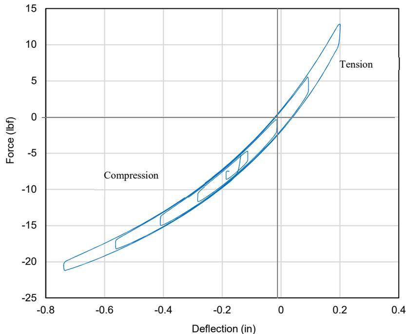
**Figure 13.** Load-deflection curve of a typical WRI in compression and in tension
