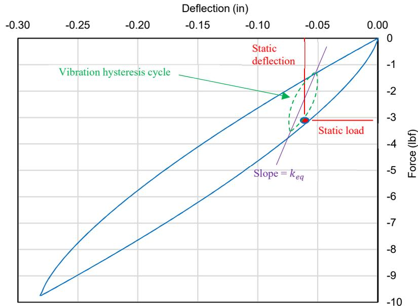
**Figure 7.** Hysteresis curve of a typical WRI in compression
