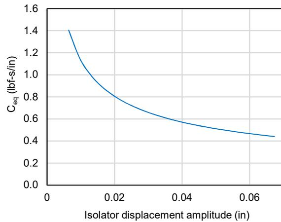
**Figure 8.**  $k_{eq}$  vs. isolator displacement amplitude for a typical WRI **Figure 9.**  $C_{eq}$  vs. isolator displacement amplitude for a typical WRI
