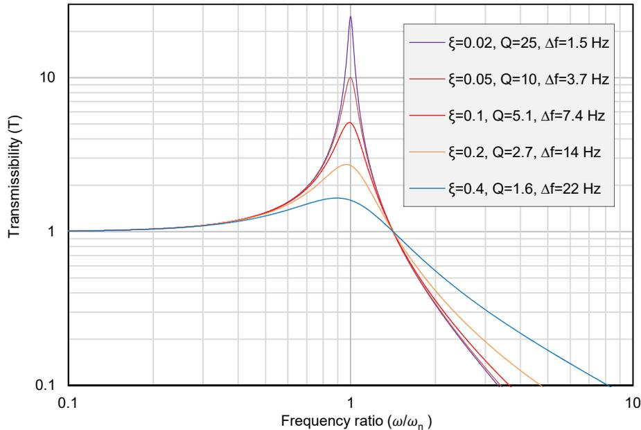
**Figure 3.** Typical transmissibility curves with varying damping ratios
