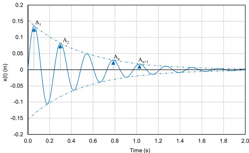
Figure 10. Post-shock free vibration of a typical underdamped, linear mass-spring-damper system
