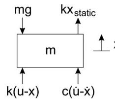
Figure 2. Free Body (FBD) of the sprung mass, m
