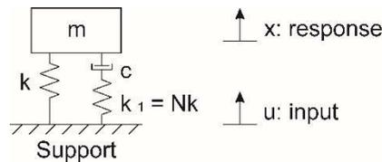
**Figure 5. Elastically connected viscous damper**
