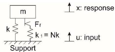
**Figure 6. Elastically connected Coulomb damper**
