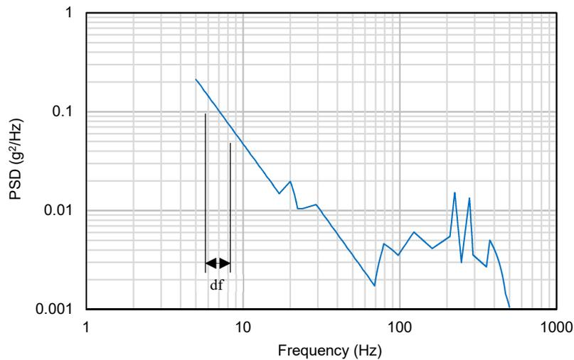
Figure 4. PSD of a typical random input signal seen on a vehicle
