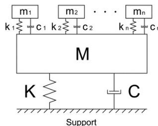
Figure 11. Model of global system, M, and its n massless critical components
