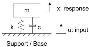
Figure 1. Mass spring damper model
