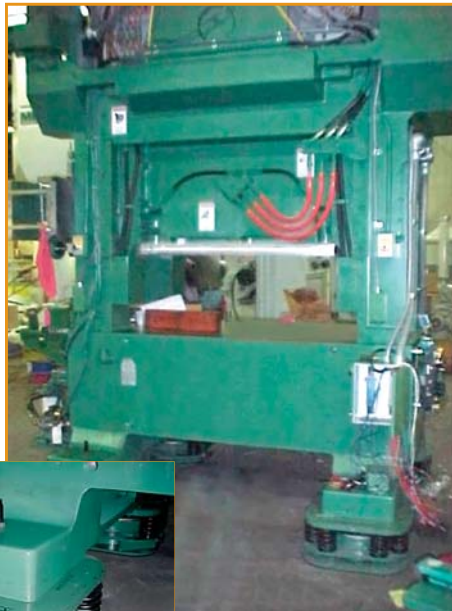
High-Speed Press on VSV Spring Isolators
