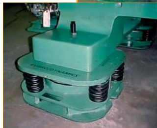
High-Speed Press on VSV Spring Isolators
