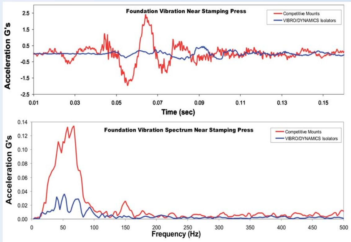
The measurements showed that the Vibro/Dynamics® Micro/Level Isolators provided an additional 80% isolation over the competitor's mounts. The customer's vibration transmission problem was solved quickly!
